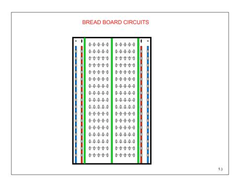
Positive lead from a battery or solar cell should be connect to the + (red) terminal. Each hole along that vertical column will be connected to that + lead.
